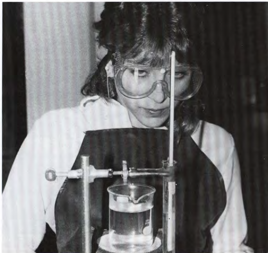
BARBARA TELLIN watches a thermometer in the test tube for decreasing changes in the temperature as the acetamide and sugar solvent start to crystalize.
