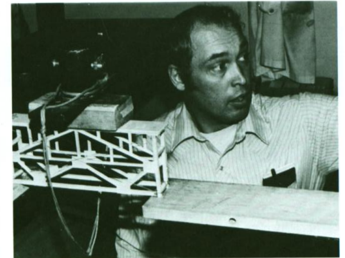
BRIDGES REQUIRED to hold at least 100 times their own weight were constructed by members of Bob Thorgesen's physics classes. Students had three days to complete structures, using only balsa wood, white glue and cotton sewing thread. The bridge above, built by Randi Grover, held 1,400 times its weight.
