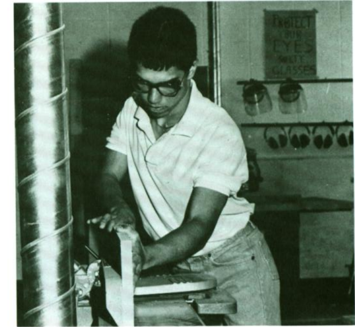
CHIPS SCATTER as Mike Coscarella uses the electric plane to level the edge of his wood. He wears safety glasses in accordance with rules requiring them when using power equipment.
